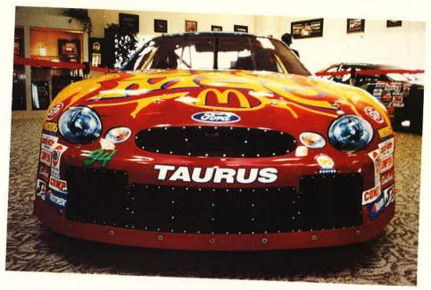
The car at the top is a short track car. Short track cars can be easily identified by the grille work, which incorporates brake ducts used to air cool brakes. The car below, which also came from the Elliott-Marino stable, is an intermediate car, which incorporates much smaller grille work. Both cars display similar aerodynamic features.
