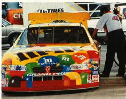
Post-race inspection calls for cars to be filled with fuel and weighed, then pushed on for more inspection.
