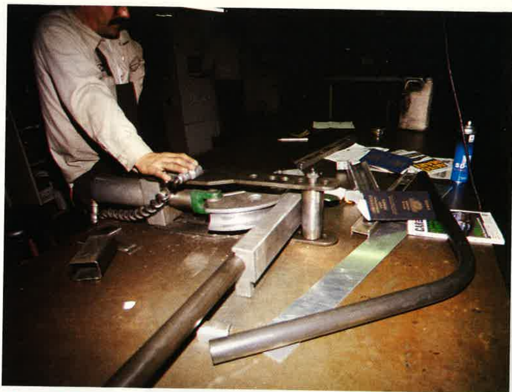
Above: Roll cages are custom bent following patterns and measurements that insure the consistency of each cage. This tubing bender is table-mounted and the fabricator is reading a scale for duplicating bends. Notice the ever-present NASCAR rule book on the bender table.
