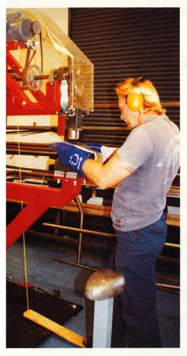
Above: Power hammers are specially designed for metal shaping and are used by many teams that find this method quicker than hammer forming or the English wheel. Above right:
