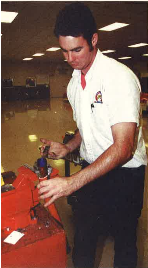
Left: This assembler is making up a braided oil line. The red covering is known as the "fire sleeve" and protects the line from outside heat sources. Vices with special jaws and precision line wrenches are used to attach "AN" style fittings to lines. Above: In this already assembled rotor and caliper, a precise fit is crucial and may require several instillation attempts to obtain the perfect fit. Assemblers know that misalignment can lose valuable tenths of seconds on the track.
