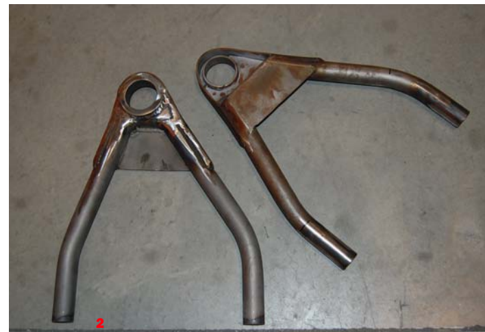
1 Before any suspension components could be fabricated, Chris Wilson and Daniel Keys had to build the custom chassis and mounts for the suspension. Here, you can see the upper and lower control arm mounts, while the coilover mounting tab is yet to be welded. 2 Here are the lower control arms in their most basic form. The guys built a fixture to ensure uniformity, but these arms are nowhere near finished. When the control arms are mounted, the guys can fabricate the coilover mounting brackets. 3 After fitting everything into place, the coilover mounts could be welded onto the flat plate on the lower control arm. A clean installation and super-clean welds are a testament to Davis' experience and the students' skill. These pieces are sandblasted and ready for powdercoating.
