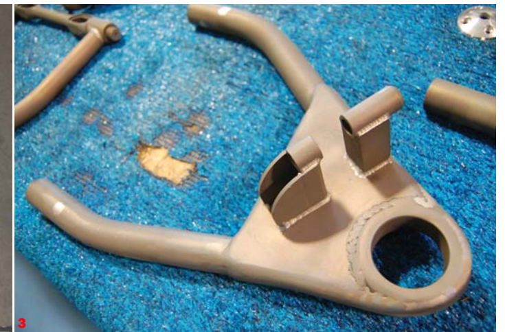
1 Before any suspension components could be fabricated, Chris Wilson and Daniel Keys had to build the custom chassis and mounts for the suspension. Here, you can see the upper and lower control arm mounts, while the coilover mounting tab is yet to be welded. 2 Here are the lower control arms in their most basic form. The guys built a fixture to ensure uniformity, but these arms are nowhere near finished. When the control arms are mounted, the guys can fabricate the coilover mounting brackets. 3 After fitting everything into place, the coilover mounts could be welded onto the flat plate on the lower control arm. A clean installation and super-clean welds are a testament to Davis' experience and the students' skill. These pieces are sandblasted and ready for powdercoating.
