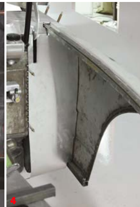
3 The panel that connects the rear floor pan to the quarter panel is held in place with Cleco fasteners for initial fit-up. It will be riveted on later. It's bead-rolled for strength and matches the shape of the adjacent panels. 4 Up front there was a similar dilemma in the aerodynamics department. Check out the cool panel that fills the void between the hand-built front fenders and firewall. This not only helps air escape from the inner fender area, but it also cleans up the car's appearance. 5 With the crush panels fabricated and installed, the crew can finish up the exhaust system with custom outlets, which will exit just in front of the rear tires. Here, a cardboard template is used to mark the steel. 6 After cutting the basic shape out of steel, the crew ties it all together with tubing, which has been cut in half. It makes for a nice curve and a strong exhaust outlet, in combination with the five vertical sleeves.
