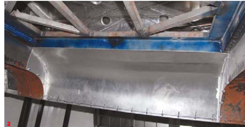
1 In the earlier stages of the build, the crew fabricated floor pans and the entire body from basic sheet steel, which left gaps between the chassis and body panels. Crush panels will fill this void and will provide awesome aerodynamics, especially at higher speeds. 2 The rear panel is pop-riveted into place. The downward roll allows air to flow off the underside of the car as smoothly as it flows off the topside. This is yet another racecar trick that Davis incorporated into the Smokin' SS Monte Carlo.
