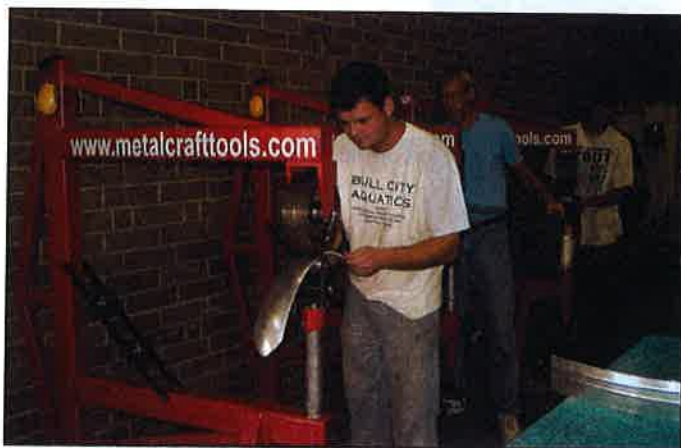
The English Wheel has been around since 1100 BC and was used for shaping armor. It is making a comeback in NASCAR Cup teams because of the fine tuning a metal shaper can put into a fender.
