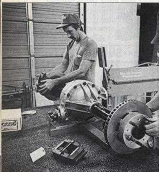
Speedway Engineering, of Sylmar, California, supplied one of its quick-change rear ends that's equipped with a Wilwood disc brake system.
