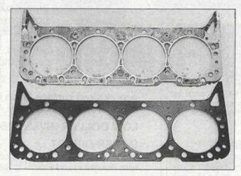
One of Jackson's tricks is to gain compression by using a special Chevrolet thin head gasket, PN 10105117. It compresses down to 0.028-inch, yielding a compression ratio of 10.7:1 for this engine, about as much as Jackson feels you can "legally" obtain given the
