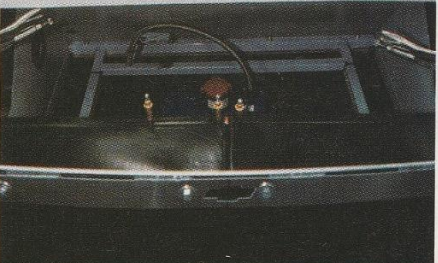
The new halo bar is a much better fit for our body. This shows how the overhead laser helps center virtually every body panel on the car. All you have to do is make sure the center of the roof panel (already marked) lines up with the laser, which tracks the car's centerline.
