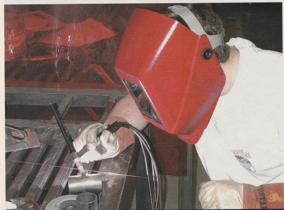
New receiver tubes for the bumpers are cut and drilled, but before they are welded to the frame, nuts are welded to the bottom side of the hole so the bolt holding the bumper tubes in place can be removed quickly with only one wrench.
