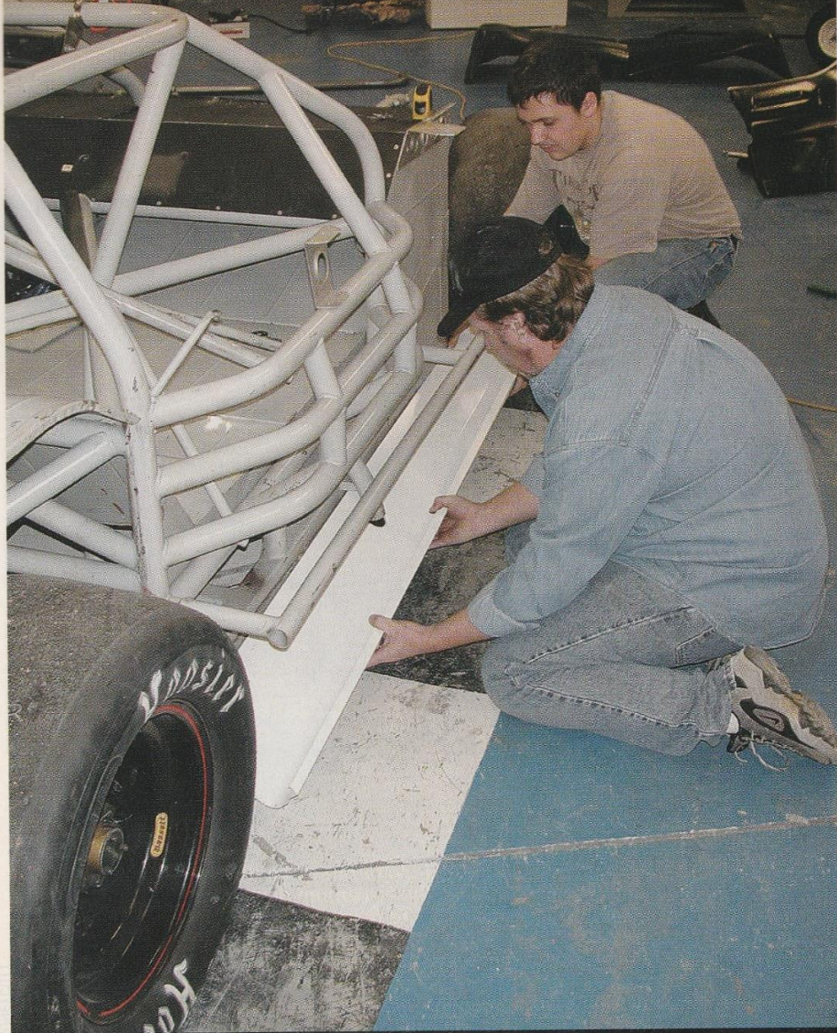
Rocker panels should follow the rake built into the frame from front to back but be parallel with the ground as they extend outward. This chassis has tabs welded to the frame for mounting rockers, but when they don't, Davis usually attaches the rockers to the bottom of the frame tubes to get them as low as possible.
