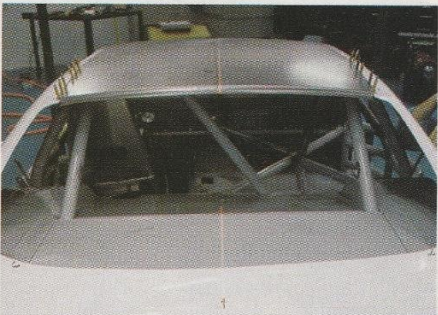
Rollcage repair may be necessary. It was in our case, so Davis had to put in the final welds.
