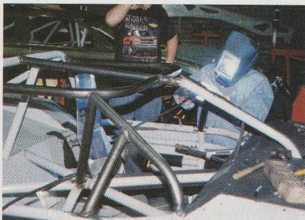
Rollcage repair may be necessary. It was in our case, so Davis had to put in the final welds.
