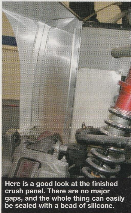
You can see the final shape of the front crush panel as Chad Dale measures off where he wants to place the pop rivets to secure the panel. A raised bead 2 inches from the edge gives the panel additional rigidity without a weight penalty.
