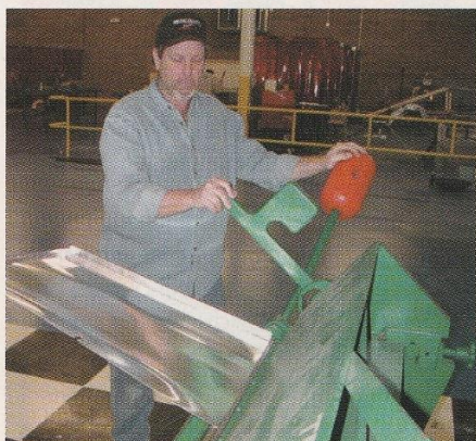
To provide strength and a place for the box's sides to be attached to the bottom, a lip is turned up on both sides with the help of a sheetmetal brake. This, of course, flattens the curves that have just been put in the sheetmetal.
