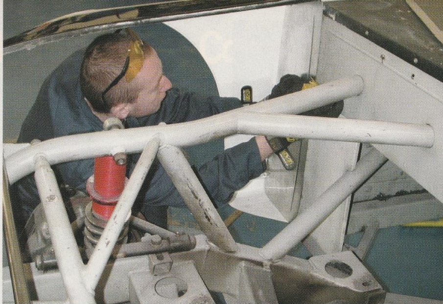
You can see the final shape of the front crush panel as Chad Dale measures off where he wants to place the pop rivets to secure the panel. A raised bead 2 inches from the edge gives the panel additional rigidity without a weight penalty.
