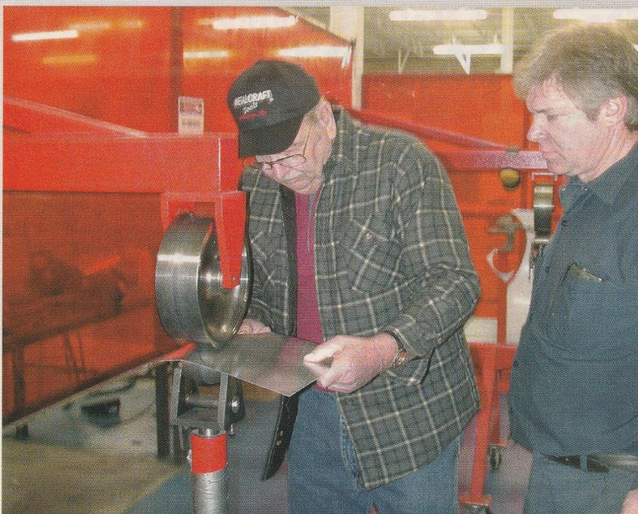
The English wheel stretches and smooths metal by compressing it between two steel wheels. Like a rolling pin rolling out dough, the wheels push metal forward causing the metal to stretch.
