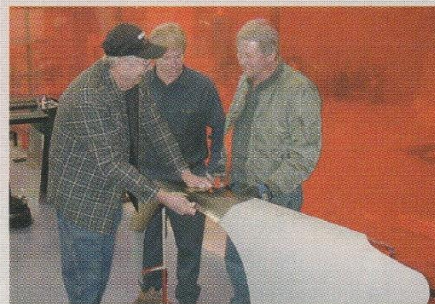
Davis (left) shows how to duplicate a fender mounted on a buck.
