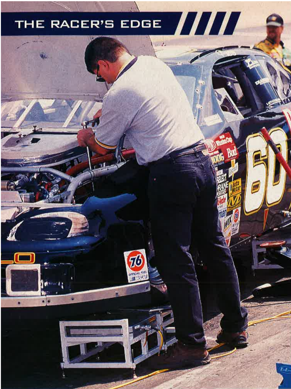
Once the car reaches the track, it is set on scales and baselined. Any changes are recorded for future use.
