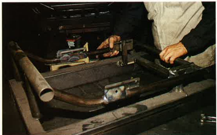
Above: The jigs are used in the placement of the roll cage on the chassis fixture. Notice that interior metal installation has started. Left: This fixture is for seat rails and seat belt brackets, later placed as a complete component in the car and welded. Left below: This lower A-arm fixture incorporates many machined parts, which, like a jig-saw, are cut and fitted to be welded as an assembly.
