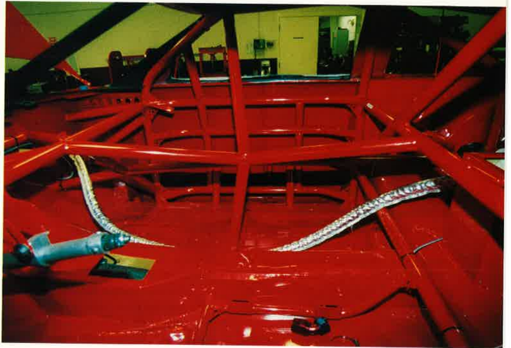
Above: A maze of brackets and bars makes painting the interior a tough job. Notice the finish is bright and slick. Left: In the prep area, skirts of masking paper control overspray.
