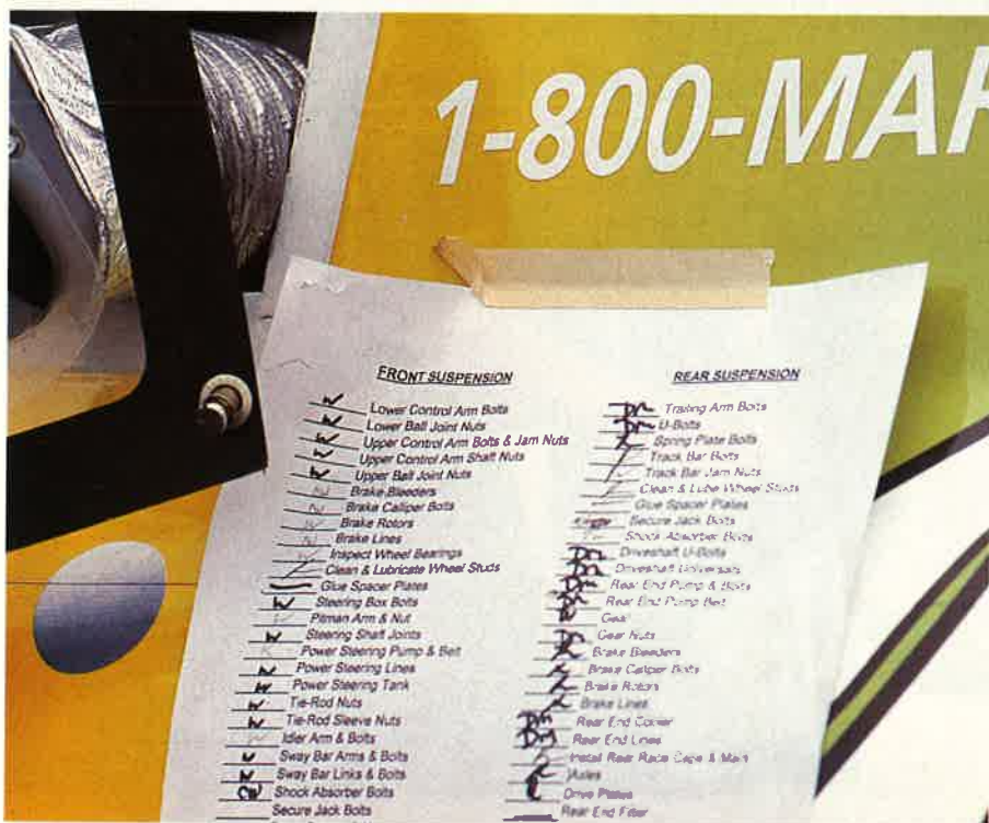
Above is an inspection list initiated by NASCAR officials. Every car has to undergo a strict NASCAR inspection before the car can circle the track on race day. Top: Springs are critical in a setup. Changes in springs alter ride height and cross weight.
